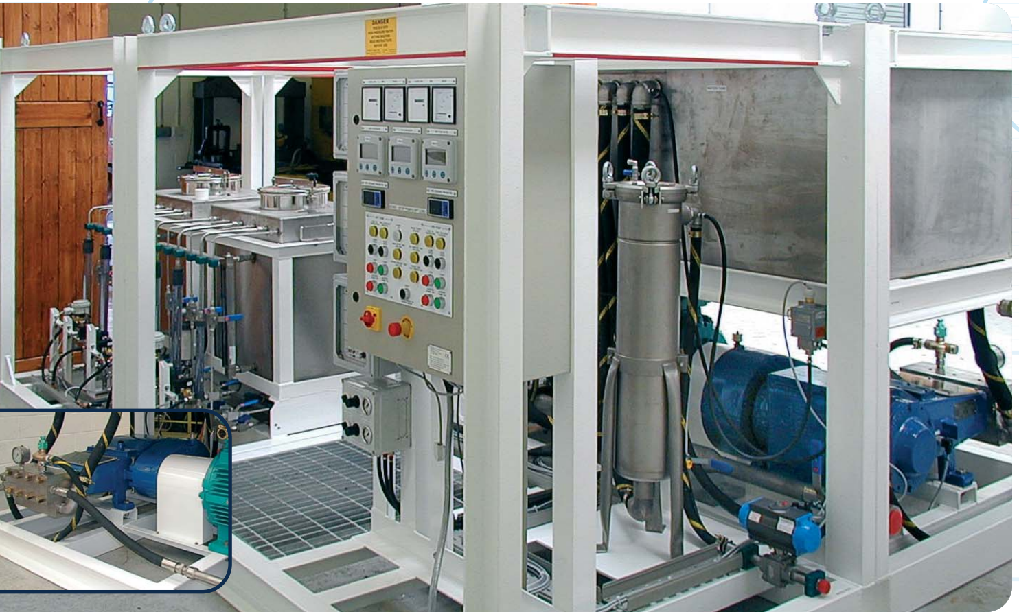
Main Picture: Subsea hydrostatic test and chemical injection system Inset: HPS2000 pump
