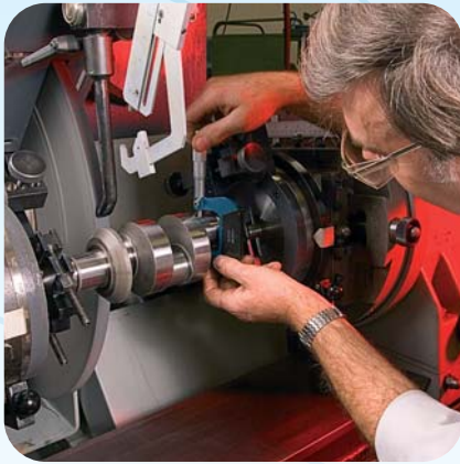
Inspection during pump crankshaft manufacture
